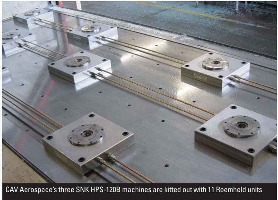
CAV Aerospace's three SNK HPS-120B machines are kitted out with 11 Roemheld units
