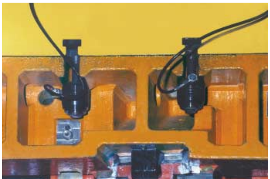
Hollow piston cylinders fastened to the press ram
