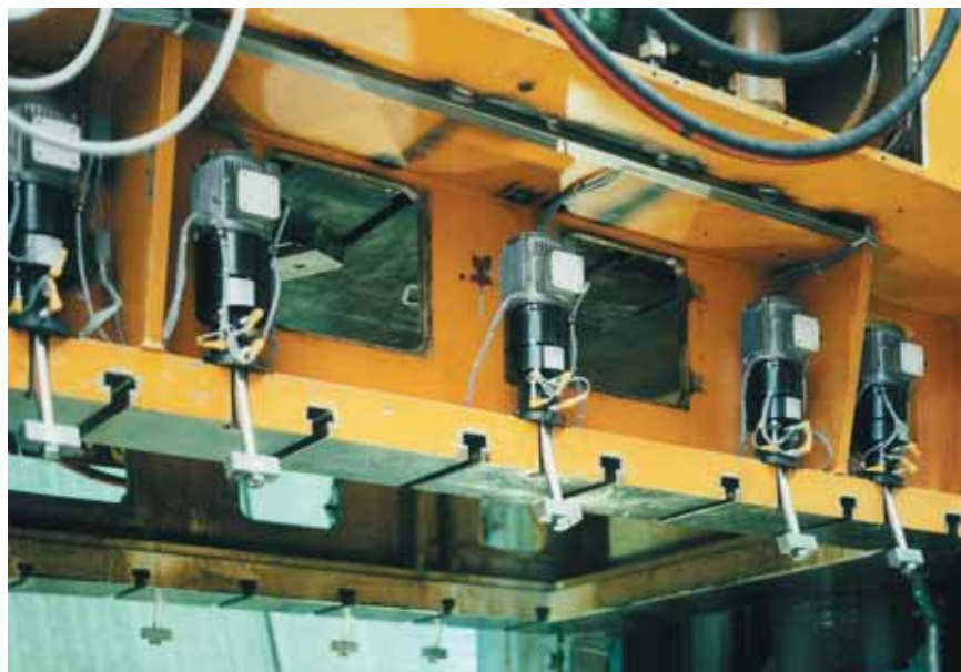
Electromechanical swing clamps mounted on a double-column press.
