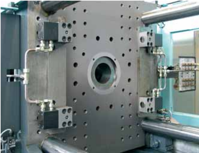
Wedge clamp on a Demag Ergotech 250/630 injection moulding machine
