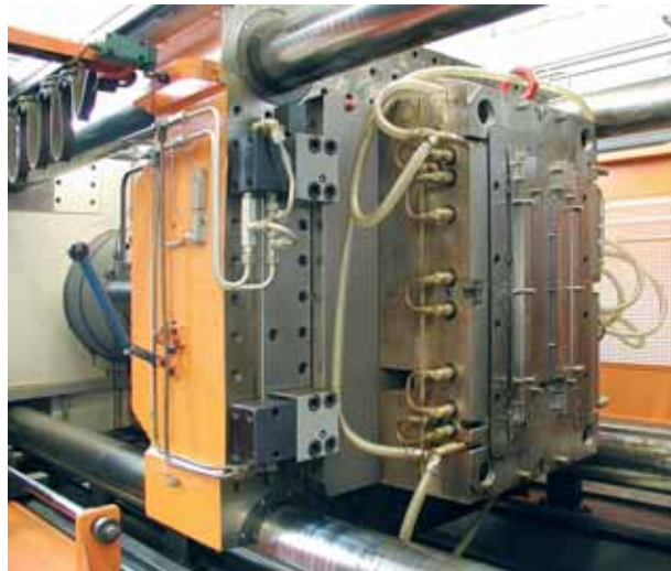
Wedge clamp with check valve on a Krauss Maffei KM 575 injection moulding machine
