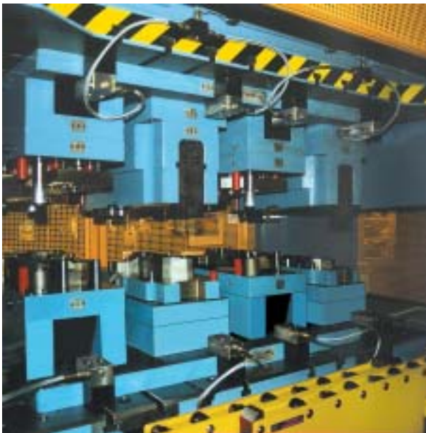
Use of sliding clamps in a double-column press, in press bed and press ram. Loading of dies using consoles (front area)
