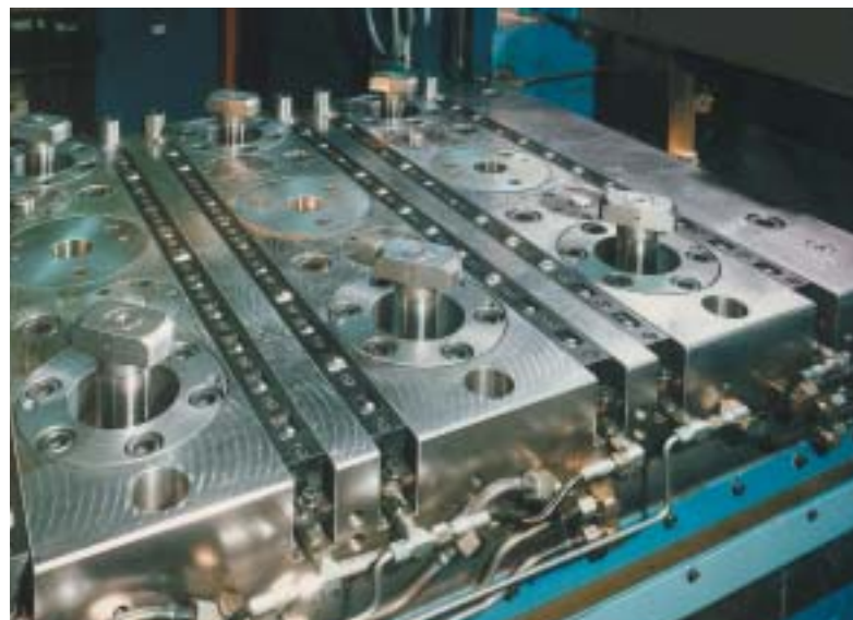
Swing sink clamps fastened in a double column press. The tie rod is extended (swing position). Easy die positioning is ensured by hydraulic roller blocs in T-slots and lateral stops
