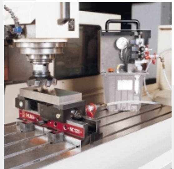
Clamping force infinitely variable on the power unit
