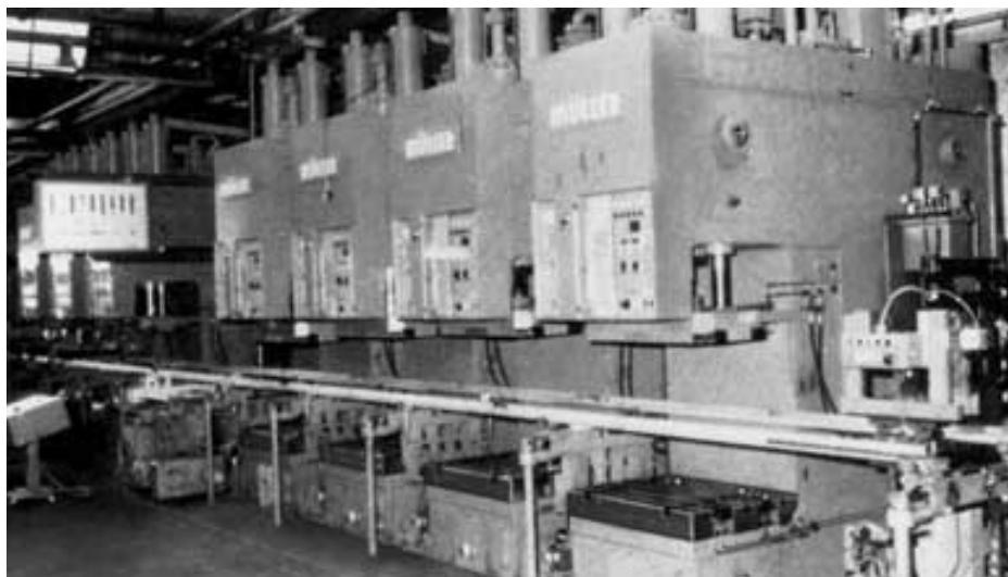
In a transfer line with seven presses the dies are clamped by means of wedge clamping elements. Monitoring system with hydraulic pressure switches.
