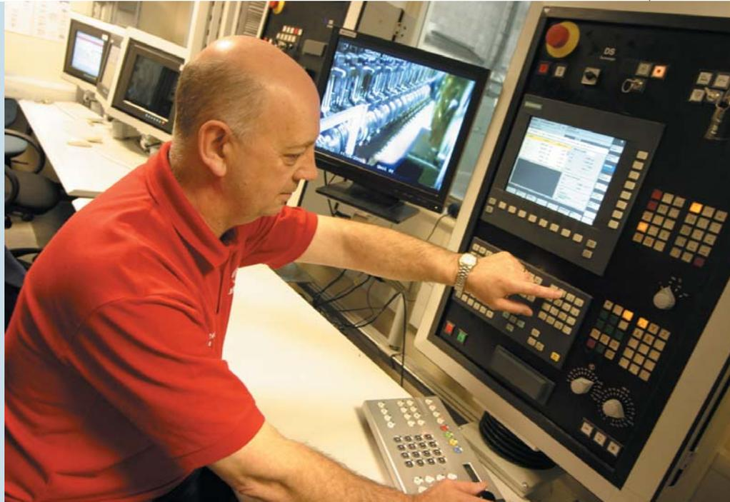
*Within the machine, and prior to any machining, cameras allow operators to inspect the clamped part to make sure it is seated/secured properly*
