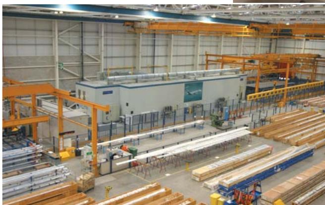
*Left, the box within a box where the DS Technologie/Roemheld system sits – extrusions are loaded from the right. Above, a stringer presented for first op, slab face machining. Right, the stringer in the lower position for second op machining, including profiling.*
